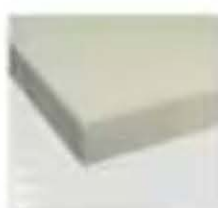
Expanded polystyrene is used for door insulation
